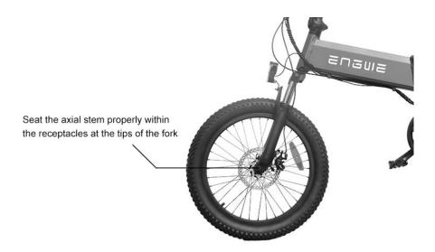
Test the brake by lifting the front of the e-bike and setting the wheel in motion (turn it) and apply the brake at the handlebar to stop it. If you could not set the wheel in free motion, or if you could not stop it by applying the brake, you need to re-adjust by increasing or decreasing the clearance.
