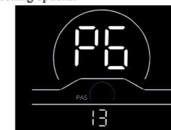
Fig. 4-6 Current Limit Setting Interface
